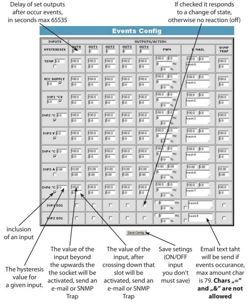
For logical input INP1D and INP2D, e-mail and SNMP Trap notification are send when input level change from 1 to 0 or 0 to 1, additional to email text (at end) will be add value 1 or 0 mark actual input state.
