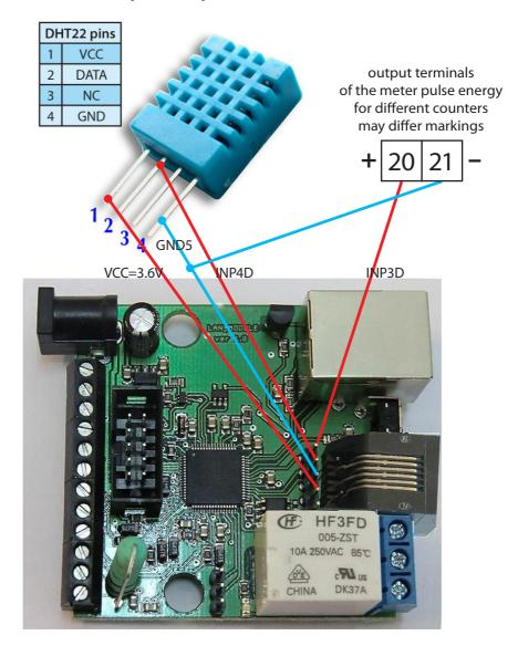
Despite of connected sensors, inputs INP4D and INP3D can still be used as a standard digital inputs in an array of events, just for the DHT11 at INP4D closed to ground will not be correct read and the shorting INP4D will calculate extra impulses.
