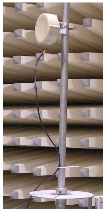
Fig. 4 measurement SXTG 5HPacD-SA (anechoic hall VUS B.Bystrica )
